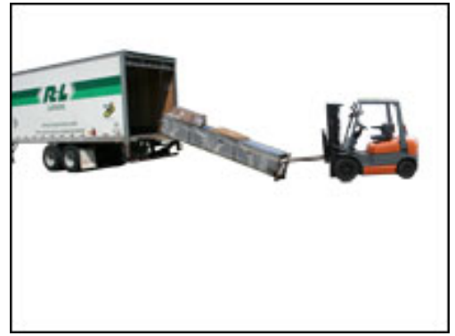
Pro Park 9 Plus 4-post lift pulled down from tailgate with fork lift.
