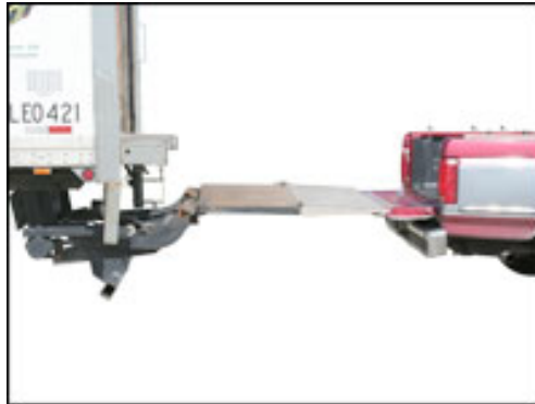
The power tailgate can be lowered to your truck's tailgate to easily off load many of our products.
